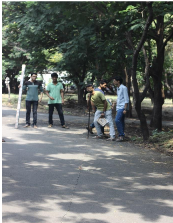
A group of B. Tech II Year Students Performing Profile Levelling Exercise using Auto-Level
